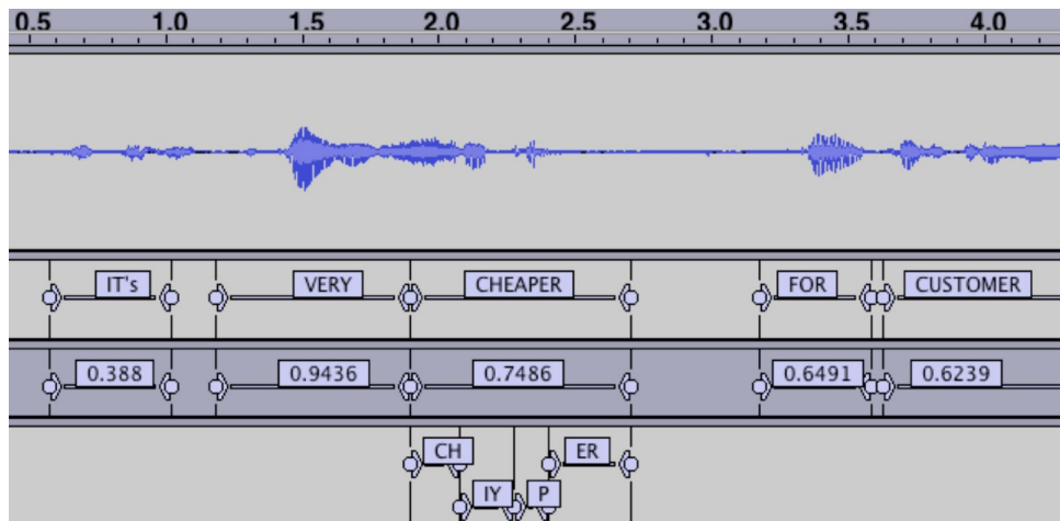
Figure 2.3: Example ASR outputs: one best sequence, phones, timestamps and word durations. Image sourced from ALTA Speech Team.
